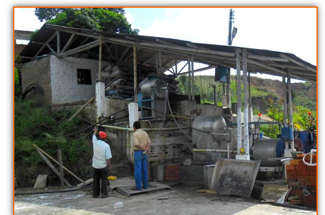
Improved rasper to increase production capacity
